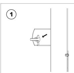
Firmly attach the carriage bolt to the pump with the nut and washer.
