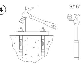
Thread nuts onto anchors, leaving approximately 1/4" of the anchor protruding, and tap into surface. **Place the 2 provided tamper-proof penta nuts on opposite sides.** Tighten nuts down to secure pump.
