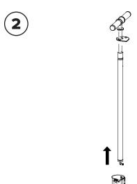
Slide the pump sideways out of the main body slot and then lift the whole pump and air lines out of the main body.
