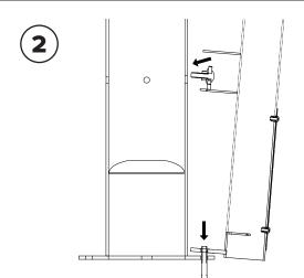
If attaching to a previously installed Fixit, remove the nut and washer on the wedge anchor on the side of the Fixit to receive the pump. Place the pump lower flange hole over the wedge anchor, and slot the previously attached carriage bolt through the hole on the side of the Fixit.
