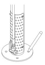
Place the Air Kit Prime in the desired location. Use a marker or pencil to outline the holes of the flange onto the base material.
