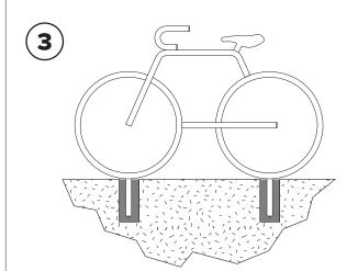
Place rack into holes, making sure the rack is level until the grout has set.
