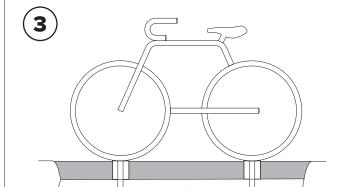
After appropriate cure time, dig out sand from sleeves and insert rack, making sure it is level and at the appropriate height. Pour in Super Por-Rok or epoxy grout and allow to set.
