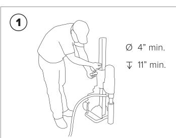
Core holes no less than 4" diameter and no less than 11" deep into sidewalk.
