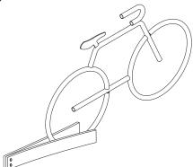
An easy way to brace the Bike Bike Rack while the grout sets is to bolt two 1x4" boards together at one end and clamp them onto the wheel of the rack like a clothes pin.
