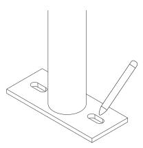
Place the rack in the desired location. Use a marker or pencil to outline the holes of the flange onto the base material.
