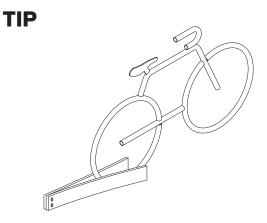
An easy way to brace the rack while the grout sets is to bolt two 1x4" boards together at one end and clamp them onto the wheel of the rack like a clothes pin.
