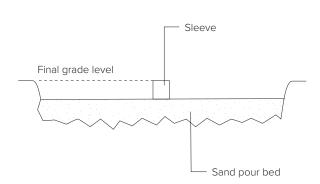
Place corrosion resistant sleeve (min. 4" inside diameter) in sand pour bed in exact location where rack will be installed. Make sure top of sleeve is at same level as desired finished concrete surface. Fill sleeve with sand to keep it in place and prevent it from filling with concrete.
