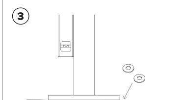
Place rack over holes, using washers to level the rack if necessary.
