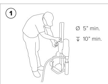
Core holes no less than 4" diameter (5" recommended) and no less than 10" deep into sidewalk.
