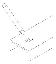
Place the rack in the desired location. Use a marker or pencil to outline the holes of the flange onto the base material.
