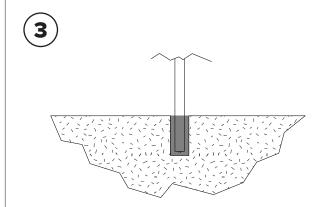
Place rack into holes, making sure the rack is level until the grout has set.
