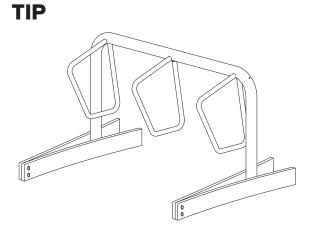
An easy way to brace the Campus Rack while the grout sets is to bolt two 1x4" boards together at one end and clamp them onto the legs of the rack like a clothes pin.
