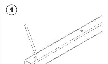
Place the rack in the desired location. Use a marker or pencil to outline the anchoring holes onto the base material.
