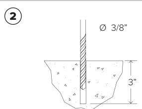
Drill 3/8" diameter holes 3" deep into surface. Make sure the holes are at least 3" away from any cracks in the base material.
