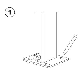
Place the rack in the desired location. Use a marker or pencil to outline the holes of the flange onto the base material.
