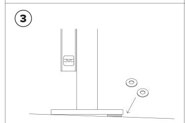
Place rack (and washers to level rack if necessary) over holes.
