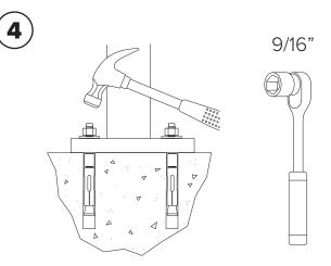
Thread nuts onto anchors, leaving approximately 1/4" of the anchor protruding, and tap into surface. Tighten nuts down to secure rack.
