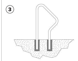
Place rack into holes, making sure it is level until the grout has set. 33"-36" of the rack should remain above the surface.
