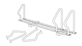
Place racks on beams so holes in rack flanges line up with beam slots
