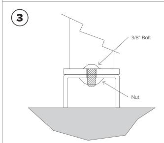
Put bolts through rack flange holes and beams so bolt head faces up. HAND tighten the nuts using new flange nuts.
