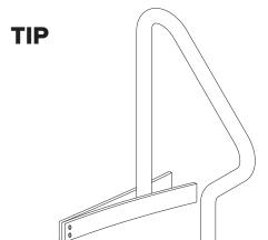
An easy way to brace the rack while the grout sets is to bolt two 1x4" boards together at one end and clamp them onto the legs of the rack like a clothes pin.
