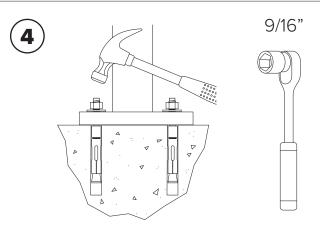
Thread nuts onto anchors, leaving approximately 1/4" of the anchor protruding, and tap into surface. Tighten nuts down to secure rack.
