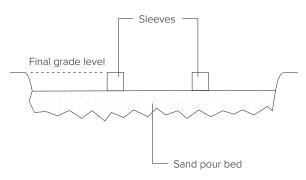
Place corrosion resistant sleeve (min. 3" inside diameter) in sand pour bed in exact location where rack will be installed. Make sure top of sleeve is at same level as desired finished concrete surface. Fill sleeve with sand to keep it in place and prevent it from filling with concrete.
