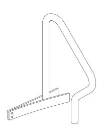
An easy way to brace the rack while the grout sets is to bolt two 1x4" boards together at one end and clamp them onto the legs of the rack like a clothes pin.
