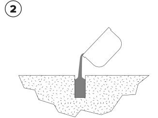
Fill holes with Super Por-Rok or epoxy grout.
