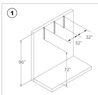
Mount 24" Slotted Tracks vertically to the wall with the appropriate anchors. Use a level for greatest accuracy. The bottom edge of the Slotted Track should be approximately 72" off the floor. The Slotted Tracks should be 32" apart from each other, and the end Slotted Tracks should be 18" from the eventual position of the end of the Trolley track.
