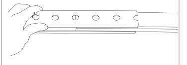
If splicing an additional length of track, slide the Splice Slotted Track over the last 6" of the 96" Slotted Track.
