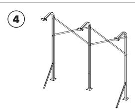
**A)** For single-sided units, attach Knee Braces to the first Upright and then every other Upright with 3/8" x 3" bolts, 3/8" washers, 3/8" lock washers, and 3/8" nuts. Anchor each Knee Brace by drilling a 3/8" hole and fastening with a wedge anchor.
