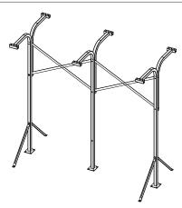
**B)** For double-sided units, attach (2) Knee Braces to the first Upright and then every other Upright with  $3/8" \times 3"$  bolts, 3/8" washers, 3/8" lock washers, and 3/8" nuts. Anchor each Knee Brace by drilling a 3/8" hole and fastening with a wedge anchor.
