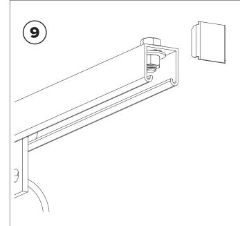
If no more Track Racks are going to be spliced together, apply hex head cap screw, washers, nut and End Cap in the open end of the Slotted Track to keep trolleys from sliding out.
