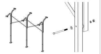
**B)** For double-sided units, fasten the Double-sided Uprights and Upright Braces to the Uprights with  $3/8" \times 3"$  bolts, 3/8" washers, 3/8" lock washers, and 3/8" nuts.
