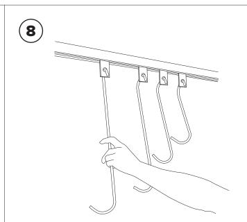
Insert the hooks through the holes in the tabs that are hanging down from the Trolleys. Each hook length should be at least 3" different than the neighboring hook.
