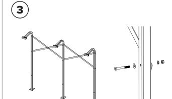
**A)** For single-sided units, fasten the Upright Braces to the Uprights with  $3/8" \times 3"$  bolts, 3/8" washers, 3/8" lock washers, and 3/8" nuts.
