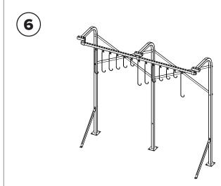
Insert the Track Rack assembly into the Channel Supports and secure. See Track Assembly instructions for more detail.
