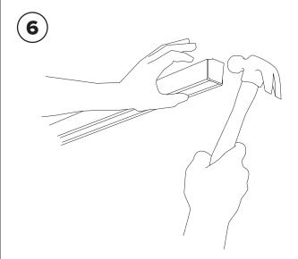
Insert a 1/2" Carriage Bolt into the last slot and fasten 3 Washers and a Tamperproof Nut. Finish by hammering in an End Cap.
