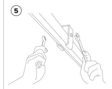
Slide Slotted Track through Channel Trolley Supports and secure in place by tightening the Hex Head Cap Screws and Flange Nuts through the holes in the Channel Trolley Supports.
