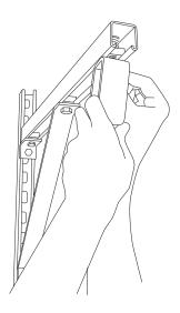
Attach the Track Rack to the Wall Mount assemblies by securing the Channel Trolley Supports to the horizontal 24" Slotted Track with the remaining Spring-loaded Nut and Hex Head Cap Screw. The edge of the Slotted Track Mounting Bracket should be flush with the edge of the 24" Slotted Track.
