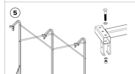
Fasten the Channel Supports to the uprights with  $1/2" \times 3"$  bolts, 1/2" washers, 1/2" lock washers, and 1/2" nuts.
