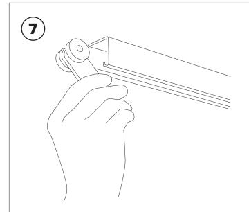
Insert the Trolleys into the open end of the 96" Slotted Track.
