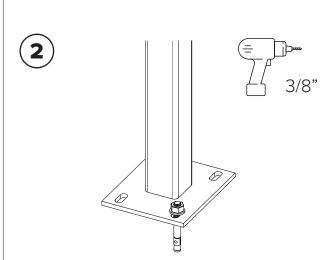
Anchor each Upright by drilling 3/8" holes and fastening with wedge anchors.
