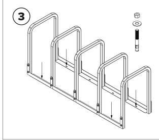
When assembly is completed, position the assembly and anchor to the ground through the slotted holes in the plates on each end of the run of racks. For longer runs you may also need to add anchors to a middle section.
