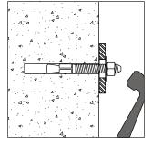
Place rack back into positon against wall and tap anchors through holes in the rack and into the
