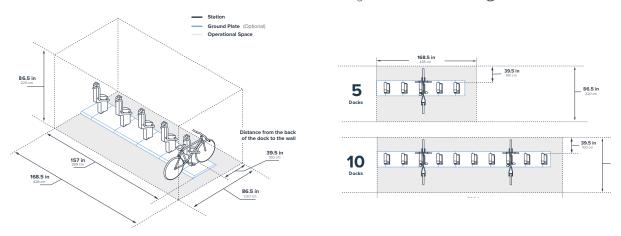
The need for Operational Space is not affected by whether the installation will be with or without Bikeep Ground Plates.
