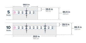
The need for Operational Space is not affected by whether the installation will be with or without Bikeep Ground Plates.
