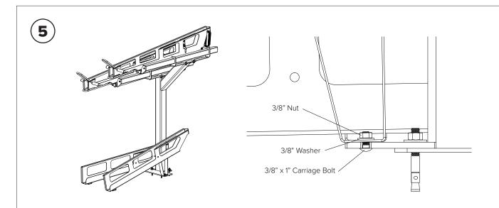
Place the bottom Lower and Upper Trays in position and secure at the rear with (1)  $3/8" \times 1"$  carriage bolt, 3/8" washer, and 3/8" nut each. Secure at the front with (1)  $3/8" \times 3"$  wedge anchor each.
