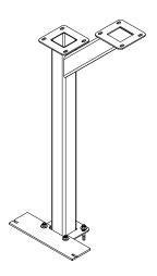
Place the Uprights in position and secure with (4)  $\frac{1}{2}$ " x 3.75" wedge anchors. At least 1.25" of wedge anchor threads should remain above the concrete. The Lower Tray Mount should be placed on the front side of the Upright and secured with the existing wedge anchors.
