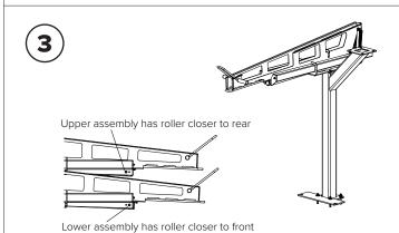
Place the lower Cantilever Assembly on the lower Upright position and secure with (4)  $\frac{1}{2}$ " x 1.25" carriage bolts,  $\frac{1}{2}$ " washers, and  $\frac{1}{2}$ " nylock nuts.
