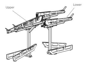
For double sided installations be sure to stagger the position of the units so that upper trays in one row face sit opposite lower trays in the other row.
