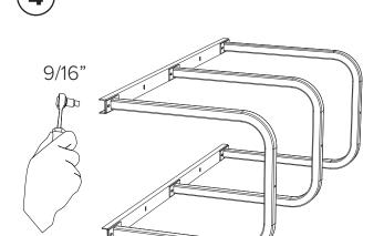
Once nuts are on, tip assembled rack over and use a 9/16" socket to tighten nuts. Before fully tightening nuts, make sure the racks are straight on beams. If using tamper resistant nuts, use access tool to tighten nuts. Do not overtighten the tamper resistant nuts. Tip rack upright.
