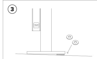
Place rack (and washers to level rack if necessary) over holes.
