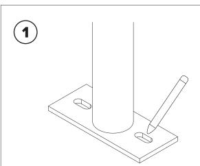
Place the rack in the desired location. Use a marker or pencil to outline the holes of the flange onto the base material.
