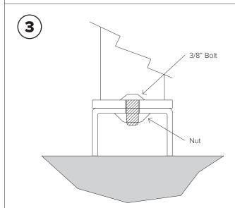
Put bolts through rack flange holes and beams so bolt head faces up. HAND tighten the nuts using new flange nuts.
