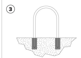
Place rack into holes, making sure it is level until the grout has set. 33"-36" of the rack should remain above the surface.
