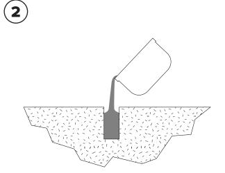
Fill holes with Super Por-Rok or epoxy grout.
