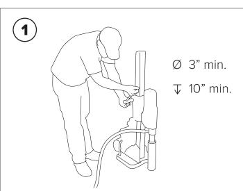
Core holes no less than 3" diameter (4" recommended) and no less than 10" deep into sidewalk.
