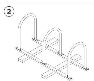
Place racks on beams so holes in rack flanges line up with beam slots
