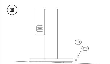
Place rack (and washers to level rack if necessary) over holes.
