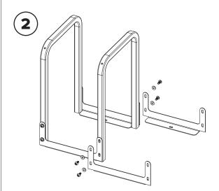
Attach the next hoop and (2) plates with (2)  $3/8" \times 1"$  tamperresistant bolts, (2)  $3/8" \times 1"$  bolts, and (4) washers. Continue attaching hoops and plates as needed.
