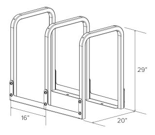
CAPACITY Single Sided: 1 bike per hoop Double Sided: 2 bikes per hoop 3 hoop minimum needed for stability **MATERIALS Hoop:** 1.5" 11g sq. tube Connectors: 11g plate **FINISHES** Galvanized An after fabrication hot dipped galvanized finish is our standard option. Pre-fabrication galvanizing is standard on panel components. **Powder Coat** Our powder coat finish assures a high level of adhesion and durability by following these steps: 1. Sandblast 2. Epoxy primer electrostatically applied
