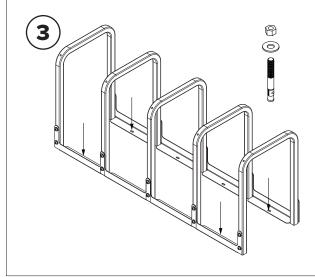
When assembly is completed, position the assembly and anchor to the ground through the slotted holes in the plates on each end of the run of racks. For longer runs you may also need to add anchors to a middle section.
