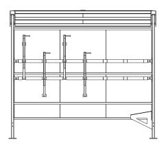
A bench may be mounted to the inside of the Pocket Shelter and still allow room for four bikes.
