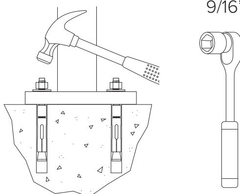
Thread nuts onto anchors, leaving approximately 1/4" of the anchor protruding, and tap into surface. **Place the 2 provided tamper-proof penta nuts on opposite sides.** Tighten nuts down to secure pump.
