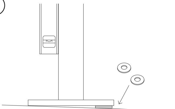
Use washers to level pump if necessary.
