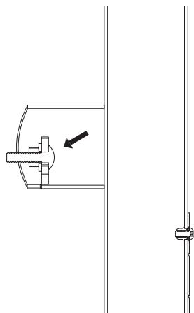
Firmly attach the carriage bolt to the pump with the nut and washer.
