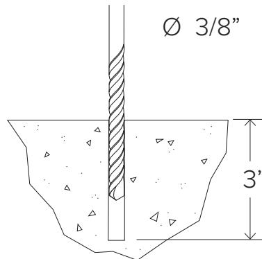
Drill 3/8" diameter holes 3" deep into surface. Make sure the holes are at least 3" away from any cracks in the base material.
