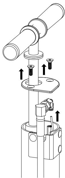
Remove the two tamper-proof screws at the top of the pump and lift the cap. Then disconnect the air line via the push-to-connect fitting at the top of the hose.
