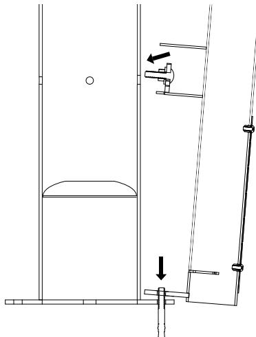
If attaching to a previously installed Fixit, remove the nut and washer on the wedge anchor on the side of the Fixit to receive the pump. Place the pump lower flange hole over the wedge anchor, and slot the previously attached carriage bolt through the hole on the side of the Fixit.
