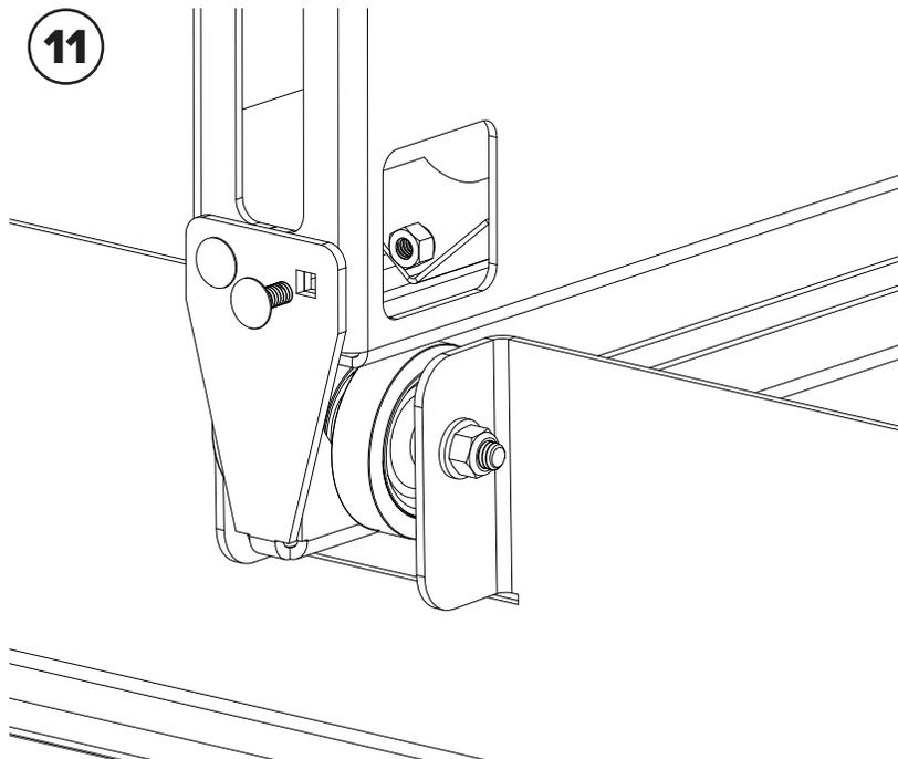
Feed the wheel guide under the center wheel and attach to the tray with (4) 1/4" x 5/8" carriage bolts and lock nuts.
