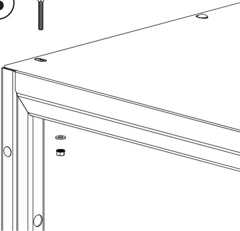
Attach the roof panels with (12) 5/16" x 2.25" carriage bolts, washers, and lock nuts. Continue adding roof panels if assembling a modular row.
