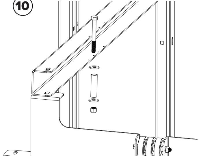
Secure the front of the (2) Dero Decker tracks with (1) 3/8" x 3.5" hex bolt, washers, and lock nut.
