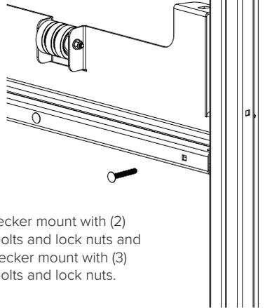
Attach the rear Dero Decker mount with (2) 5/16" x 2.25" carriage bolts and lock nuts and attach the front Dero Decker mount with (3) 5/16" x 2.25" carriage bolts and lock nuts.
