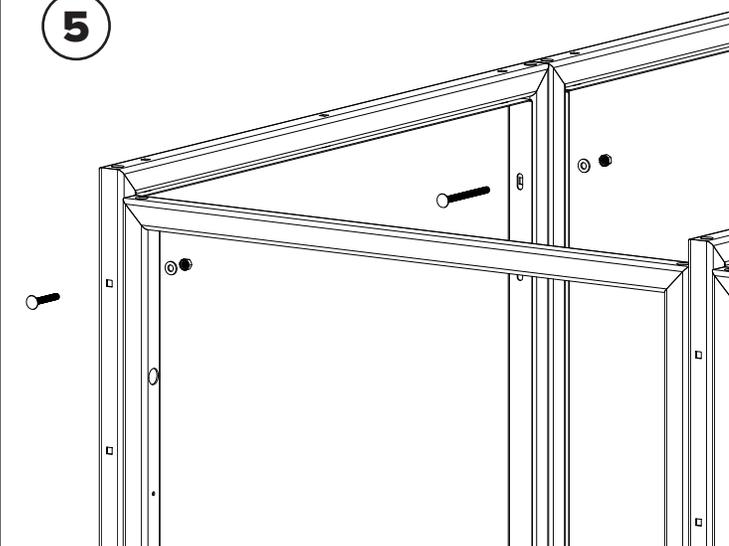
Attach the frame panels to the side positions in frame assembly with (4) 5/16" x 2.25" and (4) 5/16" x 4" carriage bolts, washers, and lock nuts. Continue adding side frame panels if assembling a modular row. The (3) bolt holes at the bottom of the panels are not used. The (3) bolt holes at the top of the panels will be used later.
