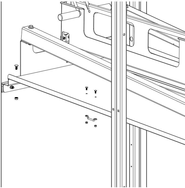
Attach the drip tray with (4) 5/16" x 3/4" carriage bolts and lock nuts. Note that the small holes in the drip tray are oriented towards the front of the locker. Attach the spring mount with (2) #10 x 1/2" carriage bolts and locknuts.
