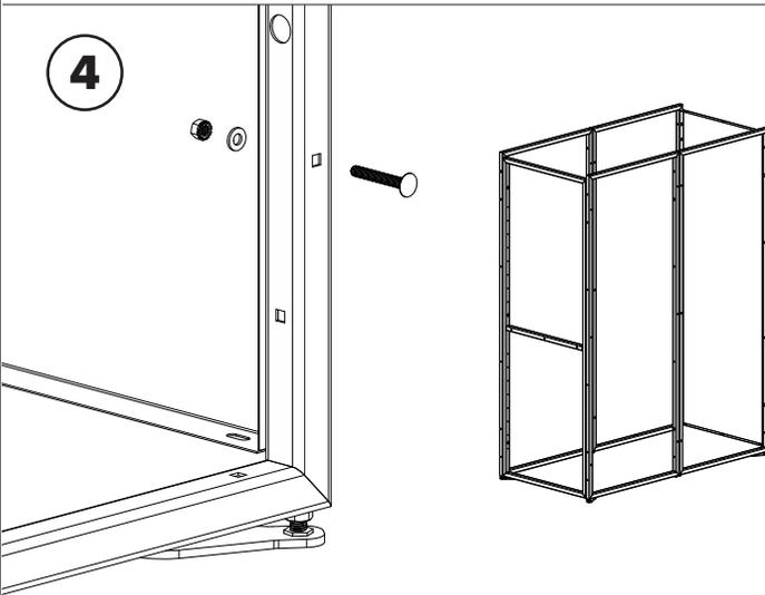
Attach (1) frame panel to the rear position in frame assembly with (4) 5/16" x 2.25" carriage bolts, washers, and lock nuts. Note the center bolt position will be left open for now. Continue adding rear frame panels if assembling a modular row.
