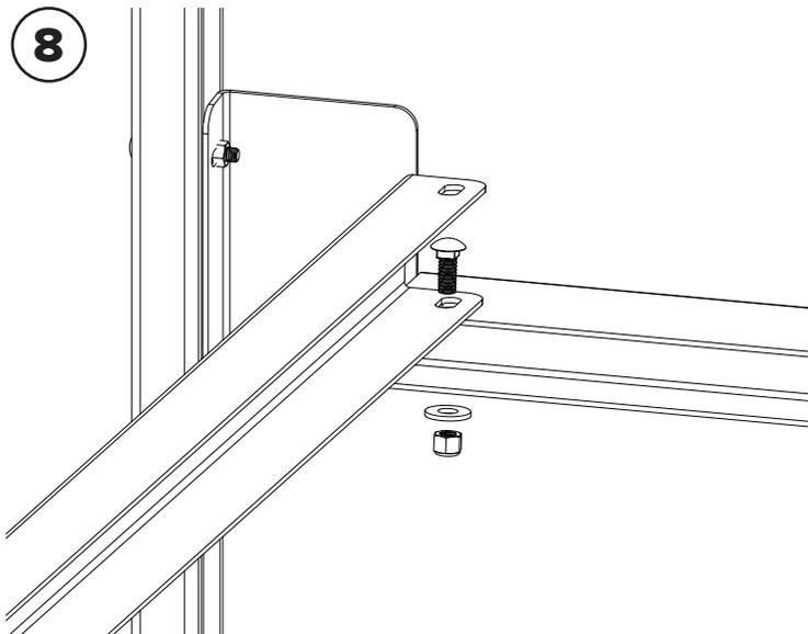
Attach the (2) Dero Decker tracks with (1) 3/8" x 1" carriage bolt, washer, and lock nut in the rear. Note the small holes in the tracks should be oriented towards the front of the locker.
