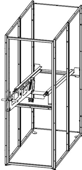
Insert the Dero Decker tray assembly into the tracks.
