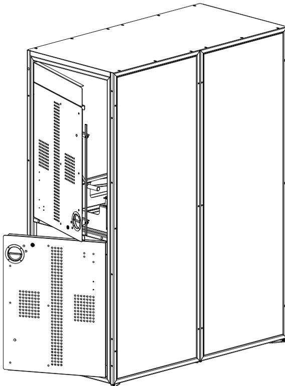
Attach the lower and upper doors with (8) #12 x 3/4" self-drilling screws. Pilot holes are present but may be partially filled with zinc. Note the upper door has an extra top panel.
