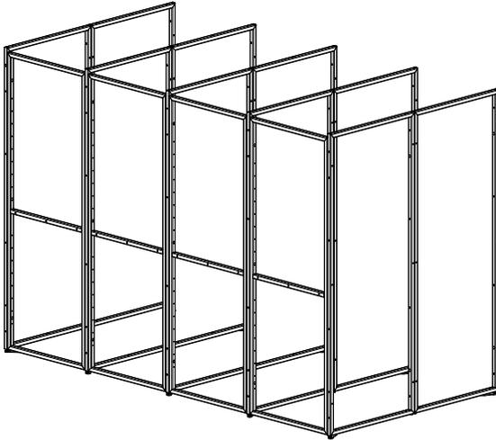
If a modular row of lockers is being assembled, continue attaching frame assemblies and door frames. Level the assembly with the leveling feet and secure them to the ground with 3/8" diameter anchors.
